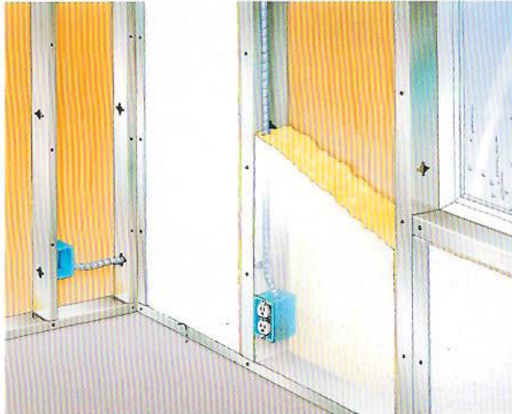
Perimeter Wall Insulation
